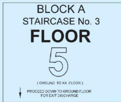
9A EXAMPLE OF A STAIRWAY MARKING SIGN [FLOOR INDICATION BOARD]
