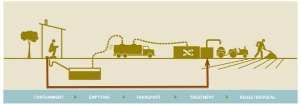
Here toilet construction technologies will ensure safe containment of human faeces from the environment Regular de-sludging of septic tanks and other on-site systems will be undertaken in a safe and scientific manner The transportation of this sludge to the treatment site shall be undertaken to approved treatment sites designated by ULBs
